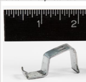
(U//FOUO) Figure 1 - AR15 Variant Component to Fire Fully Automatic
